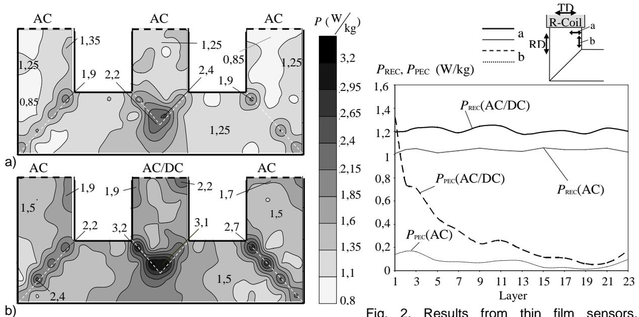
Fig. 1. Local distribution of the total losses  $P(x,y,z=0)$ . (a) Mere AC-magnetization for 1.7 T. (b) DC-bias in middle S-limb ( $r_{DC}=1.1$ ).
