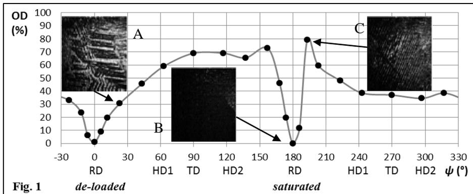
main image A for  $\psi = 20^\circ$ ). Maximum  $OD$  is reached at  $160^\circ$ . As a specific mechanism, further rotation to the saturated position  $180^\circ$  (image B) is characterized by a very sharp "jump" to  $OD = 0$ , followed then by a re-jump up to  $OD = 80\%$  (image C).
