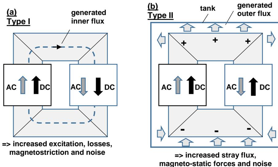
Fig.1: Two fundamental types of DC bias, illustrated for the simple case of a 2-limb 1-phase transformer core. The observed main consequences are summarized below. (a) Type 1 as causing interior flux. (b) Type 2 as causing exterior stray flux, also through the magnetic surrounding.
