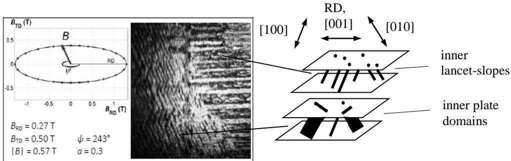
Fig. 1. A domain image under rotational magnetization for an instant when the induction vector  $\mathbf{B}$  points out near to the transverse direction (TD).
