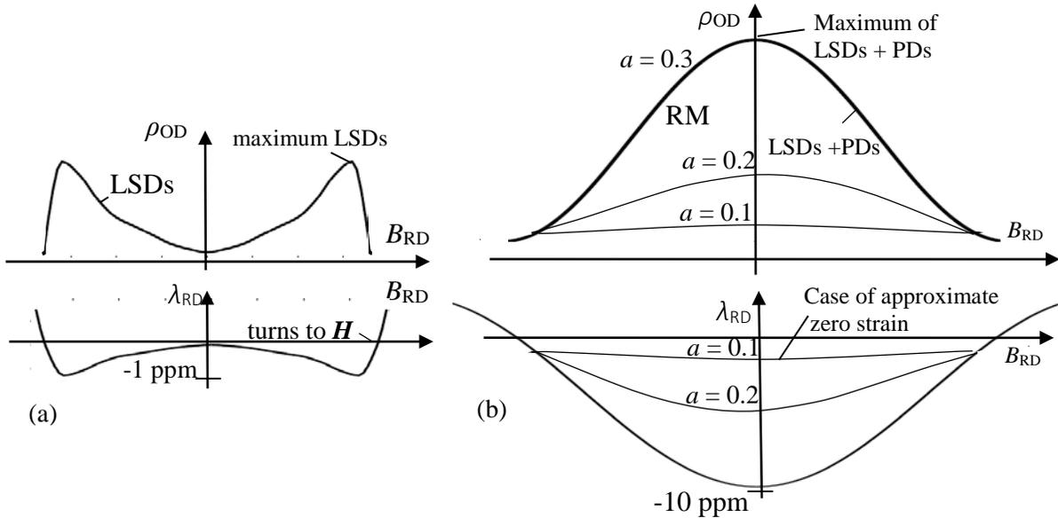
Fig. 2. A model for the volume portion  $\rho_{OD}$  of magnetic domains and the corresponding magnetostriction  $\lambda_{RD}$  in rolling direction. (a) Alternating magnetization. (b) Rotational magnetization (RM). Notice: different scale in very rough approximation for GO SiFe (see [1]).
