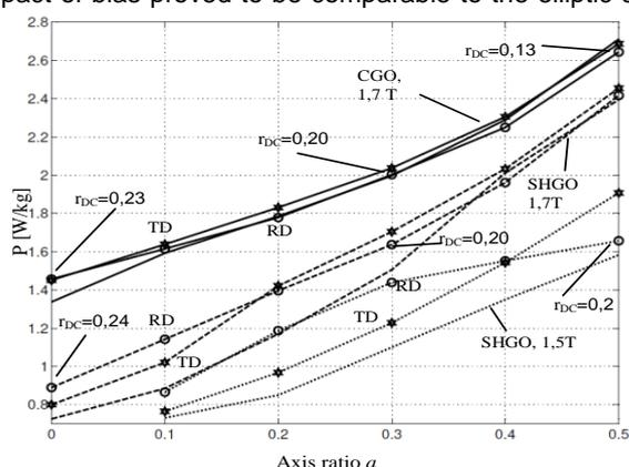
Fig.2. Losses  $P$  as a function of the axis ratio  $a$  for CGO SiFe (30M5) and for SHGO SiFe (23ZDKH90) with DC imposed in the RD and in the TD under elliptic RM. Notice that the DC/AC excitation ratio  $r_{DC}$  is not constant.
