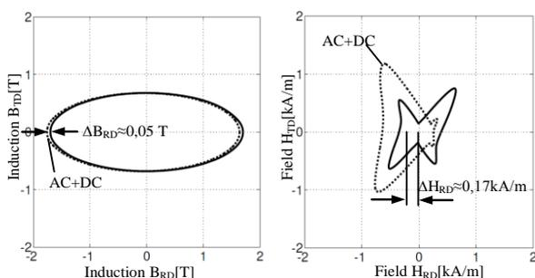
Fig.1. Example for a simulated elliptic magnetization pattern  $\mathbf{B}(t)$  with  $B_{RD} = 1,7$  T and  $a = 0,4$  of CGO SiFe. Mere AC (through lines) is compared with AC + DC in RD with  $r_{DC}$  close to 0,15 (dotted). On the right side, the corresponding field patterns  $\mathbf{H}(t)$ .
