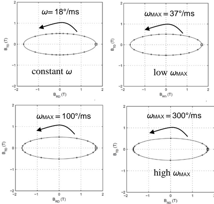
**Fig.1.** Examples for elliptic RM for  $B_{RD}=1.7$  T and  $a=0.3$  (20 instantaneous positions of the vector  $\mathbf{B}$  with time spacing of 1ms; a square for the start point). Increasing dynamics of  $\mathbf{B}(t)$  correspond to increasing maximal angular velocity  $\omega_{MAX}$  in TD. **(a)** Constant  $\omega$ . **(b)** "Even" case  $\omega_{MAX}=37^\circ/\text{ms}$ . **(c)** Practice-like  $\omega_{MAX}=100^\circ/\text{ms}$ . **(d)** High  $\omega_{MAX} = 300^\circ/\text{ms}$ .
